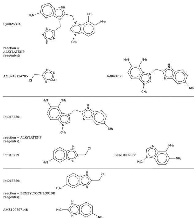
**Scheme 9** De novo design of dimers: Syn025304, the highest scoring molecule in the second *de novo* design run. The predicted stabilization energy for BEA is  $-17.5$  kJ per (mol Si), the gap with respect to the stabilization energy in BEB is  $1.5$  kJ per (mol Si).
