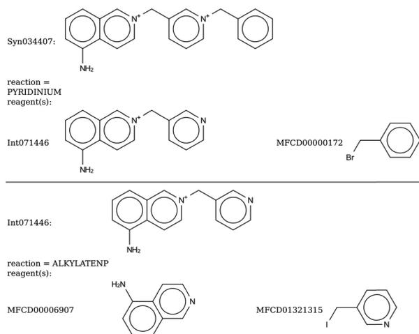
**Scheme 8** De novo design of dimers: Syn034407, the highest scoring molecule in the first *de novo* design run. The predicted stabilization energy for BEA is  $-16.8$  kJ per (mol Si), the gap with respect to the stabilization energy in BEB is  $1.0$  kJ per (mol Si).
