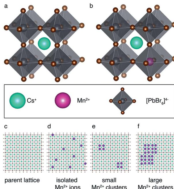
Fig. 1 Schematic representation of paramagnetic doping in perovskites: (a) parent  $\text{CsPbBr}_3$  lattice, (b) homovalent B-site replacement. Schematic representation of possible scenarios for  $\text{Mn}^{2+}$  aggregation inside the perovskite lattice: (c) parent perovskite lattice, (d) isolated  $\text{Mn}^{2+}$  ions, (e) small  $\text{Mn}^{2+}$  clusters, (f) large  $\text{Mn}^{2+}$  clusters.
