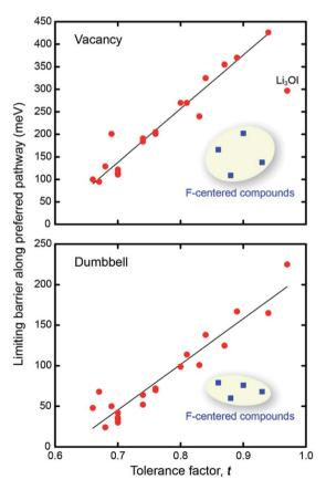
Fig. 4 Correlation between tolerance factor, t, and the limiting barrier along the preferred percolating pathway for vacancy (top) and interstitial dumbbell (bottom) migration. Blue squares depict the F-centered compounds.
