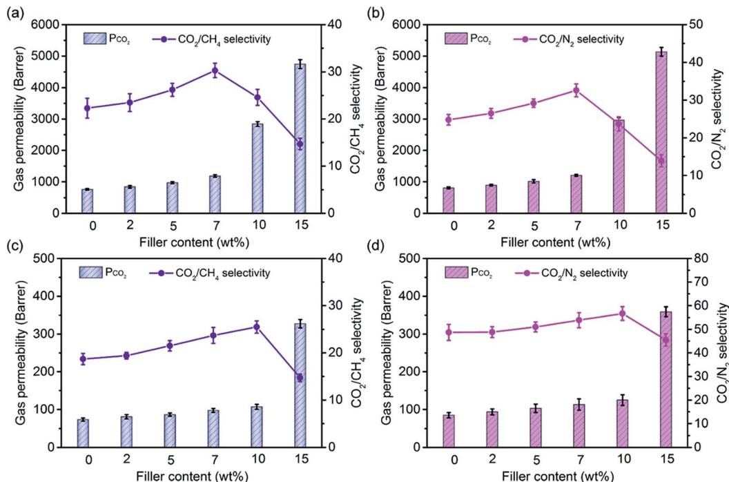
Fig. 3 The effect of the COF-300 filler content on membrane separation performance tested at 25 °C with a transmembrane pressure of 1 bar. (a) CO<sub>2</sub>/CH<sub>4</sub> and (b) CO<sub>2</sub>/N<sub>2</sub> separation performance of COF-300/6FDA-DAM series MMMs. (c) CO<sub>2</sub>/CH<sub>4</sub> and (d) CO<sub>2</sub>/N<sub>2</sub> separation performance of COF-300/Pebax series MMMs.
