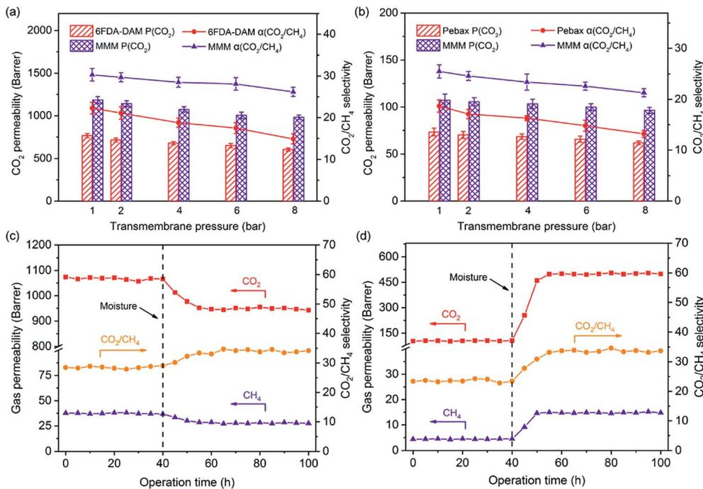
Fig. 5 Transmembrane pressure influence on the membrane  $\text{CO}_2/\text{CH}_4$  separation performance of (a) 6FDA-DAM and (b) Pebax systems tested at 25 °C. Long-term stability for  $\text{CO}_2/\text{CH}_4$  separation of MMMs in (c) 6FDA-DAM and (d) Pebax systems tested at 25 °C with a transmembrane pressure of 4 bar.
