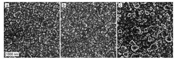
SEM micrographs of the (a) reference, (b)  $Ta_2O_5$ -overlayer, and (c) Ta-doped hematite photoanodes. The scale bar represents 1000 nm.
