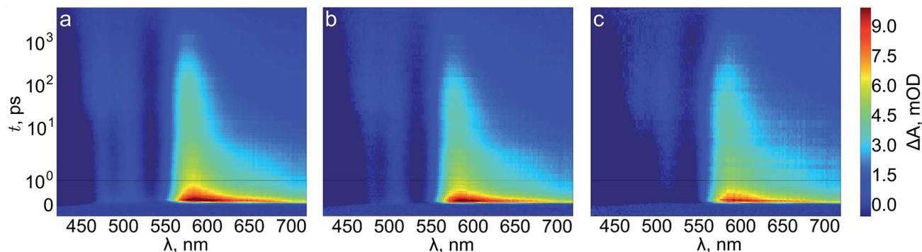
Fig. 9 Transient absorption contour plots of (a) reference, (b) Ta<sub>2</sub>O<sub>5</sub>-overlayer, and (c) Ta-doped hematite photoanodes in air.
