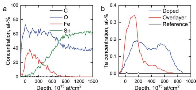
Fig. 4 (a) ToF-ERDA elemental depth profile of the reference photoanode and (b) Ta distribution in the hematite photoanodes.
