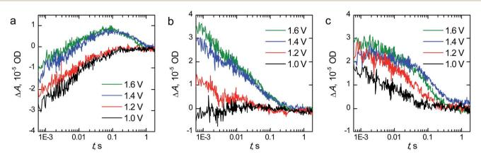
Fig. 8 Sub-millisecond to second timescale transient absorption decays at 575 nm of (a) reference, (b)  $Ta_2O_5$ -overlayer, and (c) Ta-dopedhematite photoanodes held at selected bias voltages vs. RHE.  $\Delta A$  is the change in absorbance in dimensionless optical density (OD) units.
