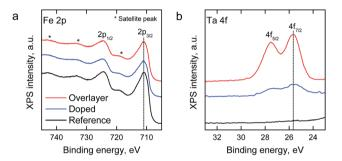
(a) Fe 2p and (b) Ta 4f XPS spectra of the hematite photoanodes.
