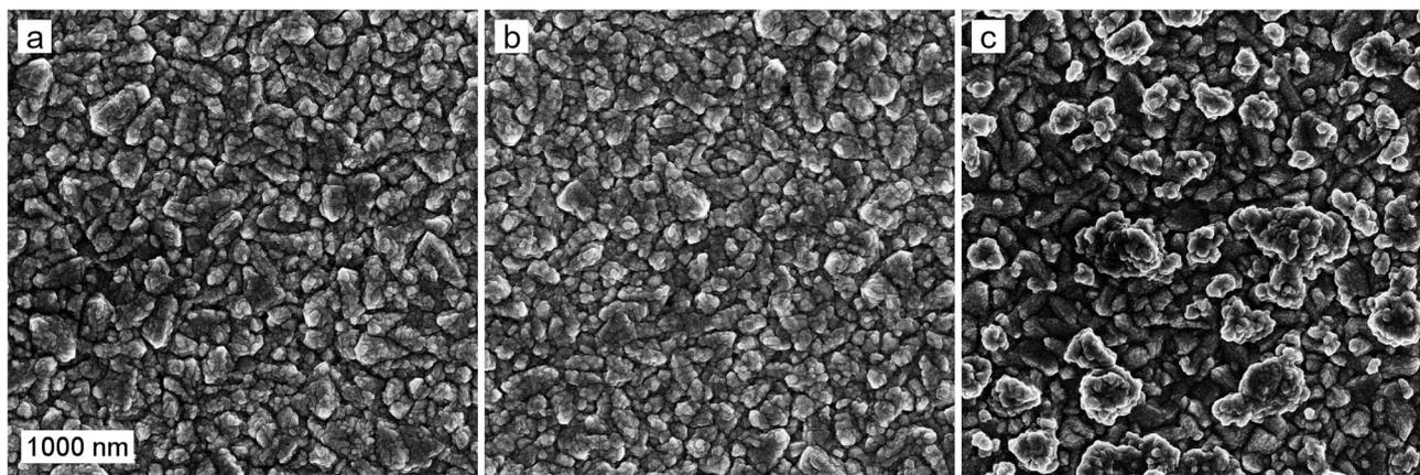
Fig. 2 SEM micrographs of the (a) reference, (b) Ta<sub>2</sub>O<sub>5</sub>-overlayer, and (c) Ta-doped hematite photoanodes. The scale bar represents 1000 nm.
