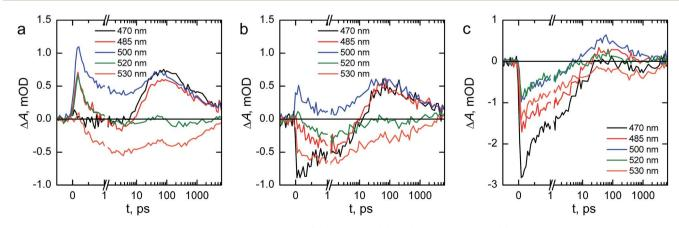
Fig. 10 Transient absorption decays at selected wavelengths of (a) reference, (b) Ta<sub>2</sub>O<sub>5</sub>-overlayer, and (c) Ta-doped hematite photoanodes in air. The timescale is linear until 1 ps and logarithmic for longer delay times.
