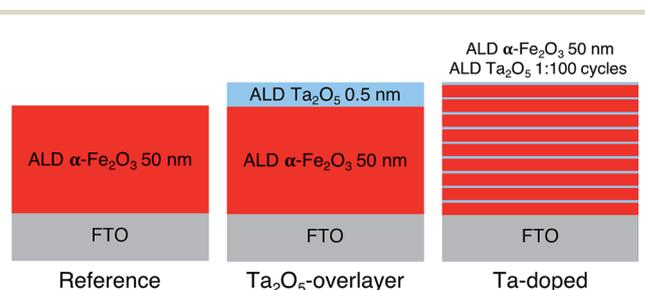
Fig. 1 Schematic representation of the ALD deposition processes for the reference, Ta<sub>2</sub>O<sub>5</sub>-overlayer, and Ta-doped hematite photoanodes.
