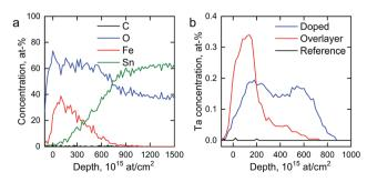
Fig. 4 (a) ToF-ERDA elemental depth profile of the reference photoanode and (b) Ta distribution in the hematite photoanodes.
