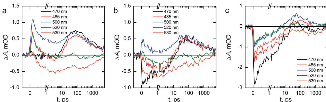
Fig. 10 Transient absorption decays at selected wavelengths of (a) reference, (b) Ta<sub>2</sub>O<sub>5</sub>-overlayer, and (c) Ta-doped hematite photoanodes in air. The timescale is linear until 1 ps and logarithmic for longer delay times.
