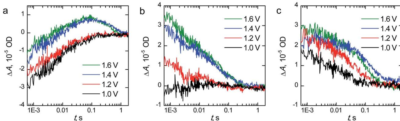
Fig. 8 Sub-millisecond to second timescale transient absorption decays at 575 nm of (a) reference, (b) Ta<sub>2</sub>O<sub>5</sub>-overlayer, and (c) Ta-doped hematite photoanodes held at selected bias voltages *vs.* RHE.  $\Delta A$  is the change in absorbance in dimensionless optical density (OD) units.
