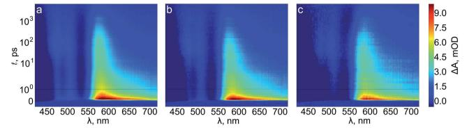
Transient absorption contour plots of (a) reference, (b) Ta<sub>2</sub>O<sub>5</sub>-overlayer, and (c) Ta-doped hematite photoanodes in air.
