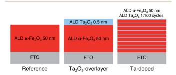
Fig. 1 Schematic representation of the ALD deposition processes for the reference, Ta<sub>2</sub>O<sub>5</sub>-overlayer, and Ta-doped hematite photoanodes.
