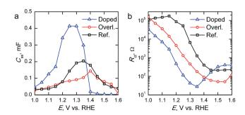
Fig. 7 (a) Surface state capacitances ( $C_{\rm ss}$ ) and (b) charge transfer resistances ( $R_{\rm ct}$ ) of the hematite photoanodes determined under 1 sun AM1.5G illumination.
