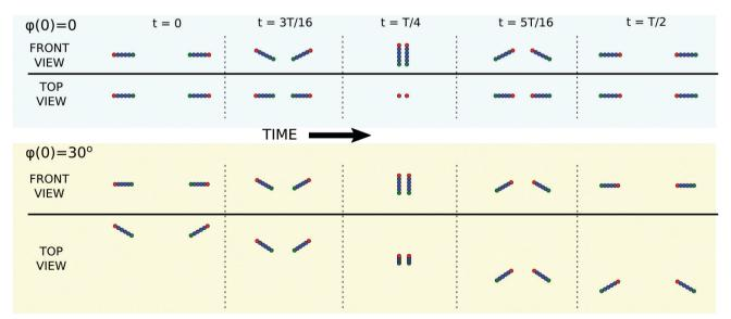
Fig. 2 Snaphots from the periodic dynamics of a symmetric pair of rods. Top panel: Quasi-2D dynamics of rods ( $\varphi(0) = 0$ ) showing tumbling motion reported before by  $Kim^{34}$  and Jung et al. 41 Bottom panel: Periodic dynamics of rods not restricted to the vertical plane (here shown for  $\varphi(0) = \pi/6$ ). Tumbling motion is combined with swinging along the 'y' horizontal axis, what is clearly visible in the top view of the system.
