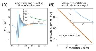
Fig. 6 Decay of the oscillation amplitude. (A) Angle  $\theta(t)-90^\circ$  as a function of time for a selected example B=10,  $\varphi(0)=45^\circ$  and  $x_{\rm cm}(0)=3$ . Dots indicate local extrema. The inset shows time intervals between consecutive extrema of  $\theta$ . (B) Exponential decay of the oscillation amplitude, the fitted relation is shown with a black line. In the inset the dependence of the amplitude ratio r is shown as a function of the filament elasticity.
