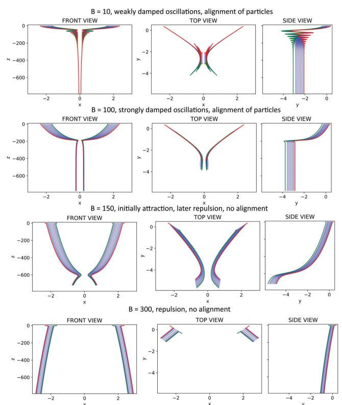
Fig. 14 Dynamics of two flexible filaments in the laboratory frame of reference, for the same parameters as in Fig. 4: N = 10,  $x_{cm}(0) = 2$ ,  $\varphi(0) = \pi/4$  and the elasto-gravitational number B as indicated. Trajectories of all the beads are shown: green and red – first and last bead of each filament, blue – other beads.
