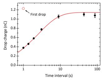
Fig. 4 Steady-state charge of a drop,  $Q_{\infty}$ , versus the time interval between subsequent drops  $\Delta t$ . The curves were fitted with eqn (21) to obtain  $\lambda$  = 5.8 mm,  $\tau$  = 6.3 s, and  $\alpha_0\sigma_L$  = 44  $\mu C$  m $^{-2}$ . 24.7 °C, 64% humidity Black points are averages of the plateaus in Fig. 3B.
