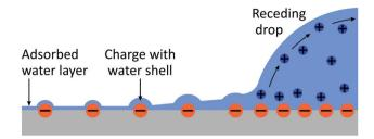
Fig. 9 Schematic of the charge transfer process.
