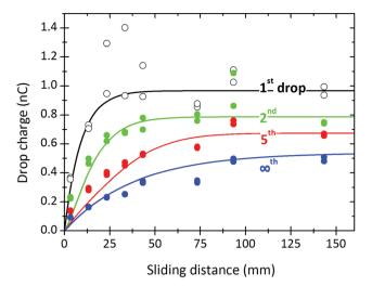
Fig. 8 Charge of the first, second, fifth drop and drops in saturation measured at different sliding lengths (symbols). Continuous lines were calculated with eqn (7), (19) and (21) using  $\lambda = 9$  mm,  $\tau = 8$  s, and  $\alpha_0 \sigma_L = 21$ , 17.5, 15, and 12  $\mu$ C m<sup>-2</sup> for the first, second, fifth and the steady state drop, respectively. 24.7 °C, 64% relative humidity. w = 5 mm,  $\Delta t = 2.13$  s. This is the same experiment as in Fig. 5.
