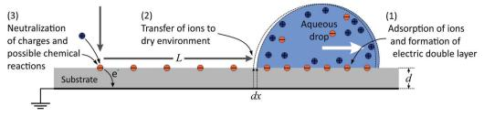
Fig. 6 Schematic of charge deposition by a sliding drop
