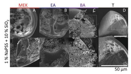
Fig. 7 SEM images of the internal microstructure of composite polymer-nanoparticle capsules obtained from droplets with initial concentration 1% w/v NaPSS + 10% w/v SiO<sub>2</sub> immersed in (A) methyl ethyl ketone, MEK, (B) ethyl acetate, EA, (C) butyl acetate, BA, and (D) toluene, T. Initial droplet radius  $R_0 \simeq$ 250-270 µm for all capsules. High magnification images of highlighted sections of the capsules are provided on the bottom row.
