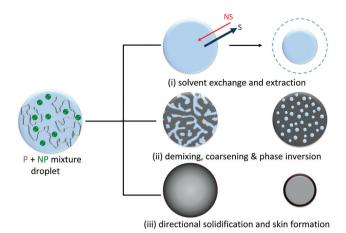
**Fig. 2** Schematic of the capsule formation mechanism, illustrating the three governing, simultaneous processes: (i) solvent exchange and extraction, resulting in drop shrinkage, (ii) droplet demixing, initiated by ingress of non-solvent, proceeding *via* spinodal decomposition or nucleation and growth, and (iii) eventual phase inversion and directional solidification, generally resulting in the formation of a smooth skin and internal microstructure.
