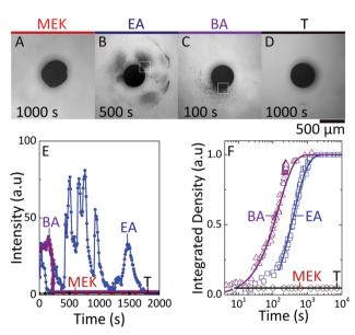
Fig. 8 Optical images of dissolution of polymer/nanocomposite capsules following immersion in DI water at pH 5-6; droplets extracted in (A) methyl ethyl ketone, MEK, (B) ethyl acetate, EA, (C) butyl acetate, BA, and (D) toluene, T, from an initial composition 1% w/v NaPSS + 10% w/v SiO<sub>2</sub>. (E) Release profile of nanoparticle clusters from marked active sites over time, and (F) overall release intensities of the respective capsules.
