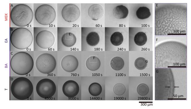
Fig. 3 Time series of solvent extraction from polymer/nanoparticle droplets with composition 1% w/v NaPSS + 10% w/v SiO<sub>2</sub> immersed in non-solvents (A) methyl ethyl ketone. MEK, (B) ethyl acetate, EA, (C) butyl acetate, BA, and (D) toluene, T. Spinodal decomposition is observed in droplets immersed in EA (E) and BA (F). Coarsening proceeds to a larger extent in droplets immersed in BA and a core-shell capsule is formed (G). The initial radius for all droplets was  $\simeq 250 \ \mu m$ .
