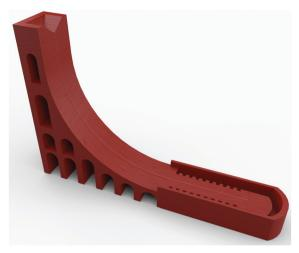
Fig. 1 Schematic of the liquid marble collision rig. The device measures  $180.8 \text{ mm} \times 30.0 \text{ mm} \times 99.5 \text{ mm}$ . A static LM is placed at the bottom of the ramp, and a second LM placed at the top. The upper LM then rolls down the ramp, colliding with the static LM. The collision is recorded at 1000 fps for analysis.
