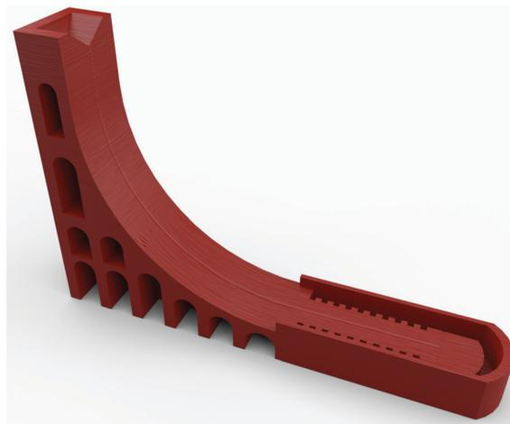
**Fig. 1** Schematic of the liquid marble collision rig. The device measures 180.8 mm  $\times$  30.0 mm  $\times$  99.5 mm. A static LM is placed at the bottom of the ramp, and a second LM placed at the top. The upper LM then rolls down the ramp, colliding with the static LM. The collision is recorded at 1000 fps for analysis.
