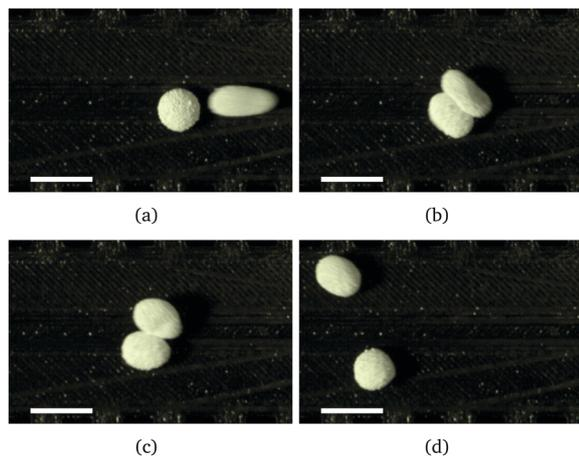
**Fig. 4** An example non-coalescing collision for  $X^* > 0.35$ . Respective time differences from frame (a) are (a) 0 ms, (b) 12 ms, (c) 17 ms, and (d) 49 ms. The mobile LM is approaching from the right. The scale bars are 5 mm. The video is available in the ESI.†
