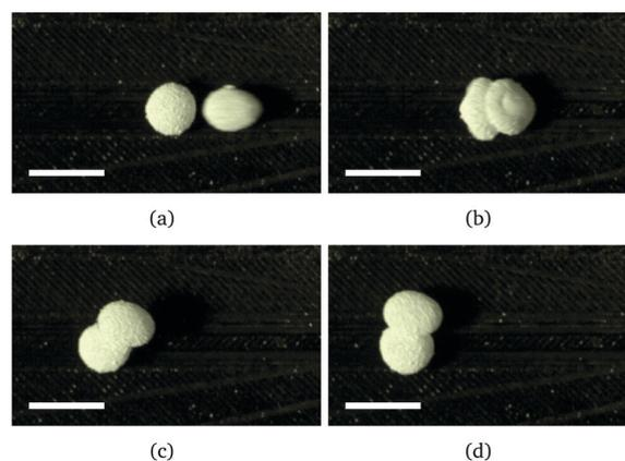
**Fig. 3** An example non-coalescing collision for  $0.05 < X^* < 0.35$ . Respective time differences from frame (a) are (a) 0 ms, (b) 7 ms, (c) 36 ms, and (d) 50 ms. The mobile LM is approaching from the right. The scale bars are 5 mm. The video is available in the ESI<sup>†</sup>.
