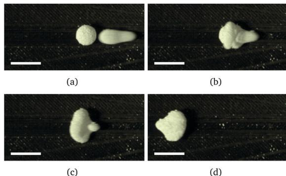
Fig. 6 An example coalescing collision for  $X^* < 0.1$  and  $\nu > 0.5 \text{ m s}^{-1}$ . Respective time differences from frame (a) are (a) 0 ms, (b) 5 ms, (c) 10 ms, and (d) 45 ms. The mobile LM is approaching from the right. The scale bars are 5 mm. The video is available in the ESI.†
