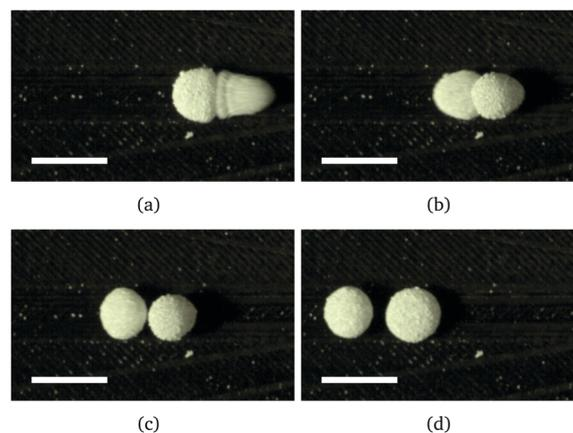
**Fig. 5** An example non-coalescing collision for  $X^* < 0.05$ . Respective time differences from frame (a) are (a) 0 ms, (b) 11 ms, (c) 32 ms, and (d) 70 ms. The mobile LM is approaching from the right. The scale bars are 5 mm. The video is available in the ESI.†
