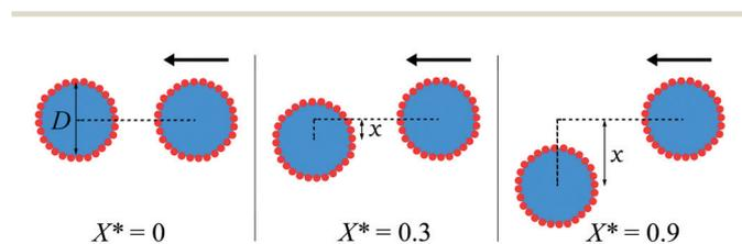
Fig. 2 Diagrams demonstrating LM collisions with offset ratios of  $X^* = 0$ , 0.3, & 0.9. The arrow indicates the direction of travel of the mobile LM. Offset ratio,  $X^*$ , is calculated by  $X^* = x/D$ ; where *x* is the distance between the centres of the two LMs, and *D* is the diameter of the LM.
