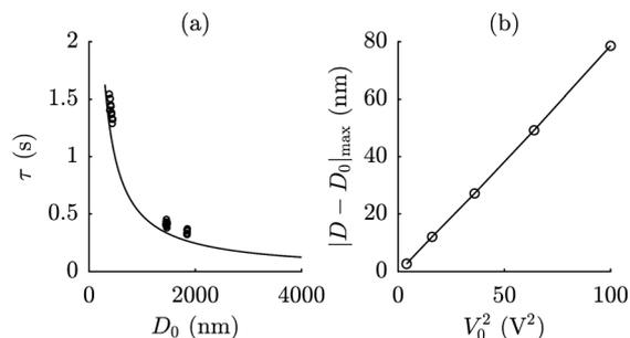
**Fig. 5** (a) Measured relaxation times (dots) in PDMS films for varying applied voltages and frequencies as a function of initial surface separation  $D_0$ , compared to the model prediction  $\tau = \gamma/k$  (solid line). (b) Measured displacement as a function of applied voltage  $V_0$ , for an initial distance  $D_0 = 3.93 \mu\text{m}$  and  $\nu_{AC} = 0 \text{ s}^{-1}$ . The displacement scales with the square of the applied voltage.
