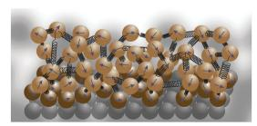
Fig. 1 Sketch of the elastomer model. Magnetic particles are depicted with an arrow representing their dipole moment and elastic constraints as springs. The lowest layer of non magnetic particles is the substrate. The darker magnetic particles laying on the substrate are the adsorbed layer, i.e., they can only move in the plane of the substrate. All other magnetic particles can move in all three directions
