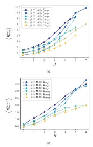
Fig. 8 Surface roughness,  $R_{rms}$ , as a function of the applied field, H, for all sampled magnetic particle densities and matrix stiffness. Symbols correspond to simulation results, dotted lines are guides to the eye. (a)  $R_{\rm rms}$ calculated from the distributions of magnetic particles only. (b) Same parameter calculated by taking into account both, magnetic particles and the volumetric particle representation of the springs described in the main text.
