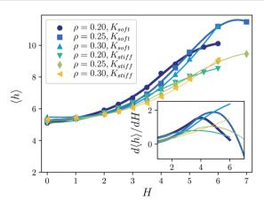
Fig. 5 Average film thickness,  $\langle h \rangle$ , as a function of the applied field, H, for all sampled densities and matrix rigidities. Symbols correspond to simulation data results, solid lines to a least squares fit of cubic splines to the simulation data. In the inset we plot the rate with which  $\langle h \rangle$  changes with H, calculated as the derivative of the fitted cubic splines.
