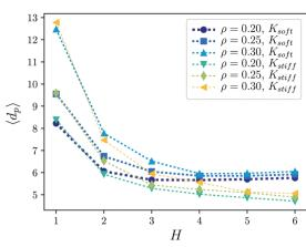
Fig. 9 Average horizontal separation between surface local maxima as a function of the applied field. Symbols represent simulation data, dotted lines are guides to the eye
