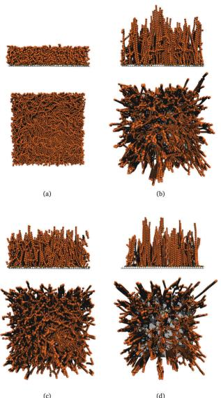
Fig. 2 Simulation snapshots obtained for selected sets of system parameters. In each panel, the top figure corresponds to the side view of the film and the lower figure to the top view. (a)  $\rho$  = 0.3,  $K_{soft}$ , H = 0. (b)  $\rho$  = 0.3,  $K_{\text{soft}}$ , H = 6. (c)  $\rho = 0.3$ ,  $K_{\text{stiff}}$ , H = 6. (d)  $\rho = 0.2$ ,  $K_{\text{soft}}$ , H = 6.
