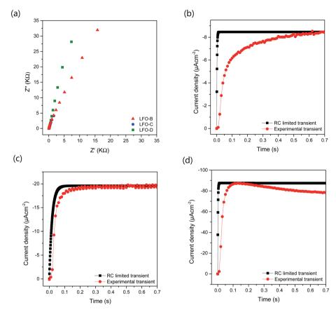
Fig. 4 (a) EIS measurements used for RC calculations in 0.1 M NaSO<sub>4</sub> with a DC of  $+0.61\,V_{RHE}$  and AC potential frequency range of  $10^5-0.1\,Hz$  with an amplitude of 5 mV under dark conditions. Experimental transient photocurrent plots from chronoamperometry measurements at  $+0.61\,V_{RHE}$  under chopped simulated sunlight with calculated RC limited transients for (b) LFO-B, (c) LFO-C, and (d) LFO-D.
