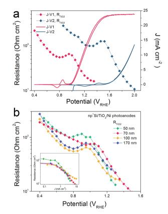
Fig. 3 (a)  $R_{\rm TiO_2}$  obtained from back contact potential (V1) and front contact potential (V2) controlled measurements. (b)  $R_{\rm TiO_2}$  thickness dependence. Inset is the  $R_{\rm TiO_2}$  as a function of the photocurrent density.
