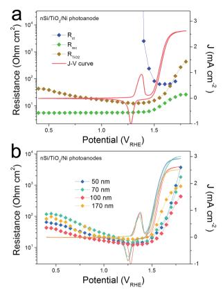
Fig. 6 (a) Resistances and photocurrent densities (*J*) *versus* the back contact potential for a  $\rm nSi/TiO_2/Ni$  photoanode. (b) CVs and  $\rm \textit{R}_{TiO_2}$  values measured from  $\rm nSi/TiO_2/Ni$  photoanodes with different  $\rm TiO_2$  thickness
