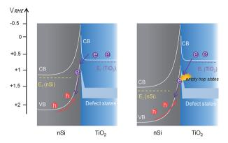
Fig. 7 Band diagram and charge transfer process at the  $nSi/TiO_2$  interface with photogenerated holes. The doping density of nSi is much smaller so that the depletion region width in nSi is very large compared to that in  $TiO_2$  (in the range of hundreds of nm), resulting in a rectifying junction.
