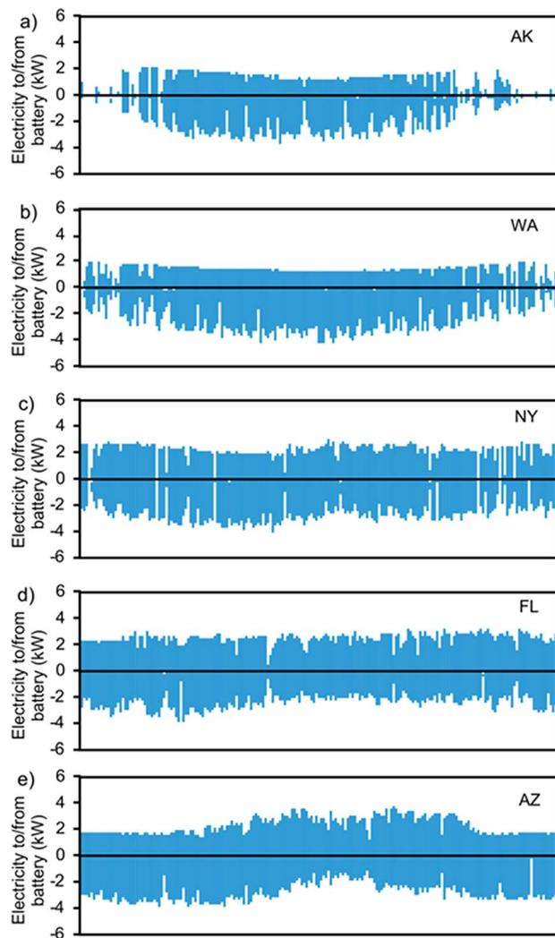
Fig. 3 Hourly power to and from the 12 kW h<sub>n</sub> battery in the five different locations: (a) Alaska, (b) Washington, (c) New York, (d) Florida, and (e) Arizona.
