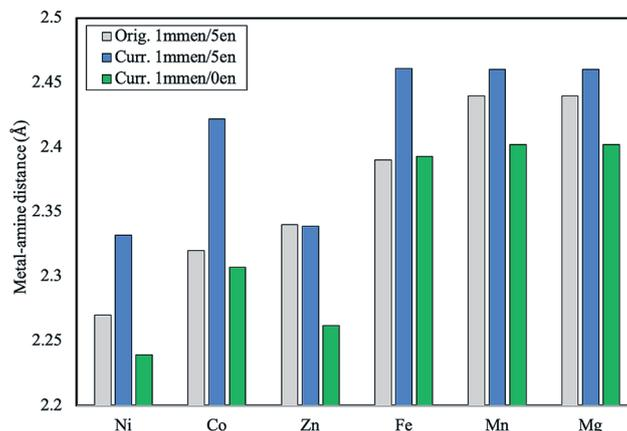
Fig. 2 Plot of the  $M-N_{\text{amine}}$  distances in Å in the original model of mmen- $M_2(\text{dobpdc})$  in comparison with the corrected numbers. Distances are reported for the structures prior to any  $\text{CO}_2$  being adsorbed.
