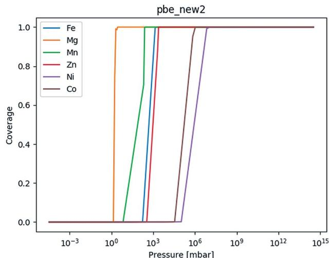
Fig. 8 The adsorption isotherm based on the chain for mmen–Mg<sub>2</sub>(dobpdc) based on the PBE values obtained as part of this erratum (Table 5).
