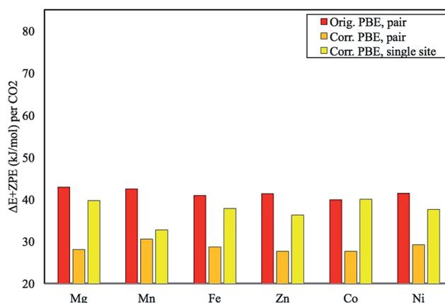
**Fig. 4** Plot of the original pair model  $\Delta E + ZPE$  in  $\text{kJ mol}^{-1}$  in comparison with the corrected numbers. The results for the first step in pair formation, a single-site CO<sub>2</sub> binding energy, are also given. Energies are reported per CO<sub>2</sub> adsorbed.
