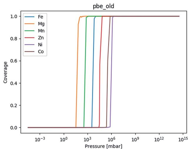
Fig. 7 The adsorption isotherm based on the chain for  $\text{mmen-Mg}_2(\text{dobpdc})$  based on the PBE values in the original manuscript.
