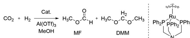
Scheme 1 Reductive transformation of CO<sub>2</sub> towards the formaldehyde oxidation level yielding methyl formate (MF) and dimethoxymethane (DMM).
