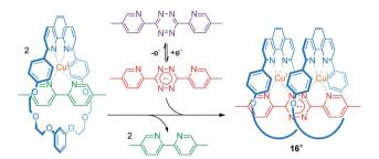
Fig. 13 Electrochemical switching of a multi-component system to reversibly form the palindromic pseudo[3]rotaxane 16<sup>+</sup>.
