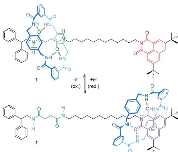
Fig. 2 Electrochemically switchable molecular shuttle **1**. In the neutral state, the tetralactam wheel preferably encircles the diamide station. One-electron reduction to the **1**<sup>-</sup> state moves the wheel to the naphthalimide radical anion site.
