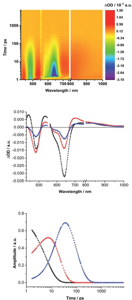
Fig. 6 (Top) Differential absorption spectra obtained by femtosecond transient absorption pump-probe experiments (550 nm, 400 nJ) of  $(\text{TCBD-aniline})_3\text{-SubPc(TCBD-aniline)}$  **2** ( $3 \times 10^{-5}$  M) in argon-saturated anisole with several time delays between 1 to 7500 ps. (Middle) Deconvoluted evolution associated spectra and (bottom) associated time-dependent amplitudes obtained *via* global analysis in GloTarAn monitoring formation and decay kinetics.
