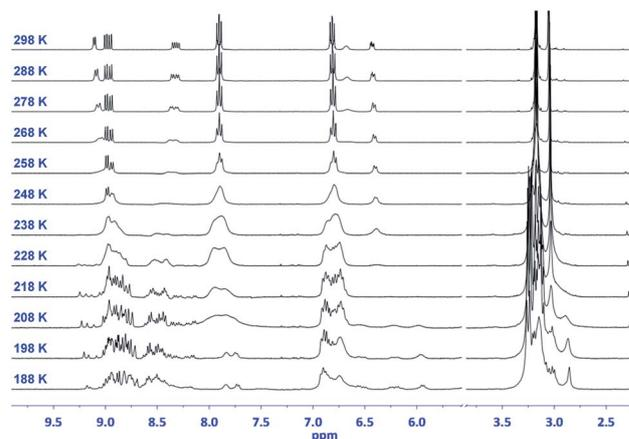
Fig. 2 Variable-temperature <sup>1</sup>H-NMR spectra (CD<sub>2</sub>Cl<sub>2</sub>) of (TCBD–aniline)<sub>3</sub>-SubPc(TCBD–aniline) **2**.
