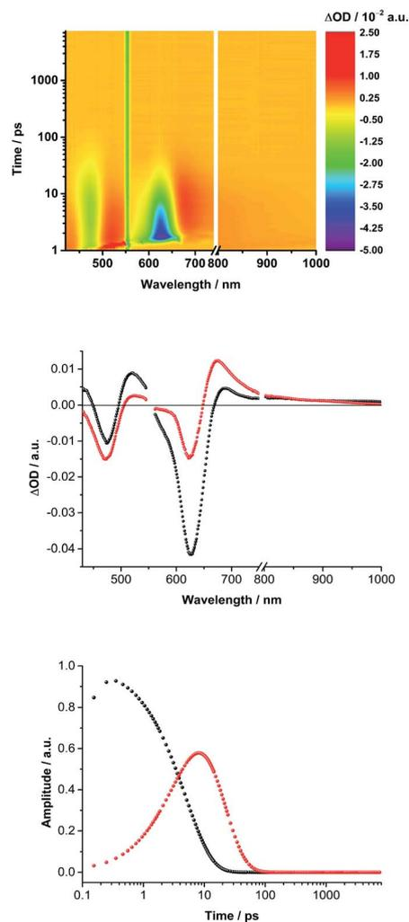
Fig. 4 (Top) Differential absorption spectra obtained by femtosecond transient absorption pump-probe experiments (550 nm, 400 nJ) of (TCBD-aniline)<sub>3</sub>-SubPc(<sup>t</sup>BuPhO) **1** ( $2 \times 10^{-5}$  M) in argon-saturated anisole with several time delays between 1 to 7500 ps. (Middle) Deconvoluted evolution associated spectra and (bottom) associated time-dependent amplitudes obtained *via* global analysis in GloTarAn monitoring formation and decay kinetics.
