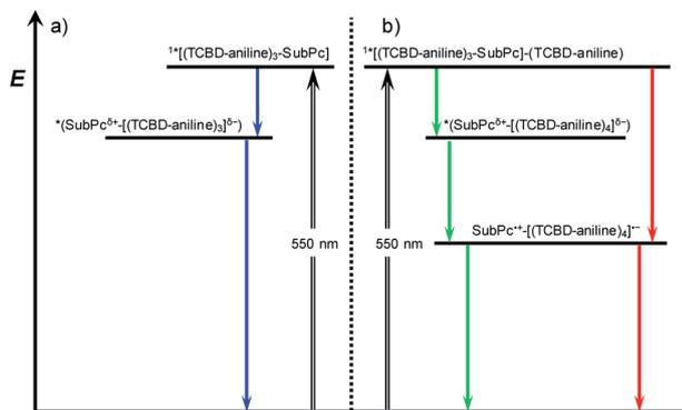
Fig. 5 Energy level diagram of (a)  $(\text{TCBD-aniline})_3\text{-SubPc}$  ( $^t\text{BuPhO}$ ) **1** in toluene, chlorobenzene, anisole, and benzonitrile (blue arrows) and (b)  $(\text{TCBD-aniline})_3\text{-SubPc(TCBD-aniline)}$  **2** in chlorobenzene and anisole (green arrows), and benzonitrile (red arrows) reflecting the energetic pathways after excitation of SubPc ( $\lambda_{\text{ex}} = 550$  nm, black arrow). Blue, green, and red arrows refer to nonradiative processes.
