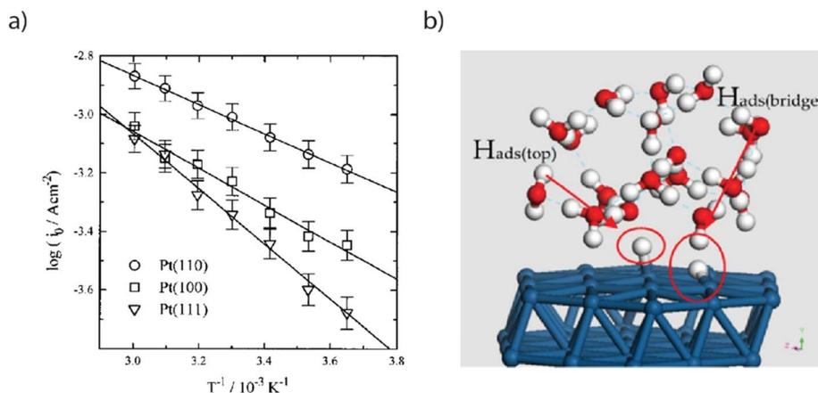
Fig. 2 (a) Arrhenius plot of exchange current densities for Pt(110) (circle), Pt(100) (square) and Pt(111) obtained by cyclic voltammetry in a 50 mM H<sub>2</sub>SO<sub>4</sub> solution (reproduced from ref. 21 with permission from the American Chemical Society, Copyright (1997)). (b) Snapshot of a MD-DFT simulation showing the presence of two types of adsorbed hydrogen on a Pt(111) electrode. Reproduced from ref. 23 with permission from Elsevier, Copyright (2007).
