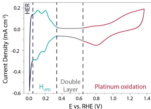
Fig. 1 Cyclic voltammogram recorded on a Pt(pc) electrode at 50 mV s<sup>-1</sup> in a 0.5 M H<sub>2</sub>SO<sub>4</sub> solution degassed with argon.
