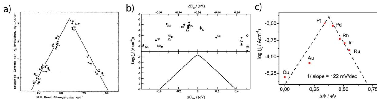
Fig. 3 Dependence of the exchange current density of the HER on the (a) measured (reproduced from ref. 26 with permission from Elsevier, Copyright (1972)) and (b) calculated (reproduced from ref. 23 with permission from Electrochemical Society, Inc., Copyright (2005)) metal hydrogen binding energy and (c) difference of work-function between a hydrogenated and a wetted surface (reproduced from ref. 28 with permission from PCCP Owner Societies, Copyright (2017)).
