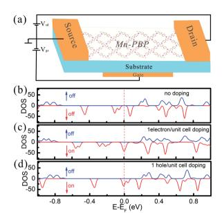
Fig. 5 (a) The schematic of a spin-field-effect transistor device based on Mn-PBP. (b) The total DOS of spin-up and spin-down electrons without electron/hole doping. The total spin-up and spin-down DOS of Mn-PBP with (c) one electron or (d) one hole doped per unit cell.
