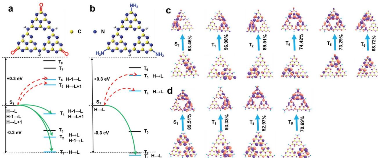
Fig. 4 Schematic representations of the TD-DFT calculated energy levels, main orbital configurations, and possible ISC channels of (a) W-CNQDs, and (b)  $g\text{-C}_3\text{N}_4$  in the singlet ( $S_1$ ) and triplet ( $T_n$ ) states. H and L refer to the HOMO and LUMO, respectively. Diagrams showing NTOs (hole orbitals on the bottom and electron orbitals on the top) and the corresponding proportions for (c) W-CNQDs and (d)  $g\text{-C}_3\text{N}_4$ .
