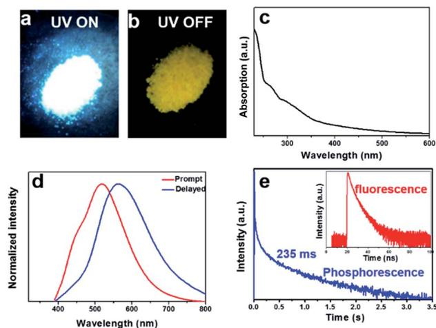
Fig. 3 Photographs taken before (a) and after (b) the UV light (365 nm) is turned off. (c) The UV-vis absorption spectrum. (d) Prompt (red line) and delayed (blue line, 5 ms) PL spectra, excited under 380 nm. (e) Time-resolved decay spectra measured at 520 nm for long lifetime and at 440 nm for short lifetime (inset) of W-CNQDs.
