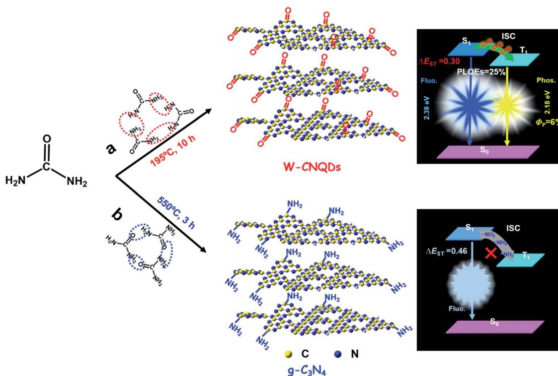
Fig. 1 A schematic diagram showing the preparation and energy-level diagrams of the relevant photophysical processes of (a) W-CNQDs and (b)  $g\text{-C}_3\text{N}_4$  ( $\Delta E_{ST}$  = energy gap,  $S_0$  = ground state,  $S_1$  = singlet excited state,  $T_1$  = triplet excited state, ISC = intersystem crossing).
