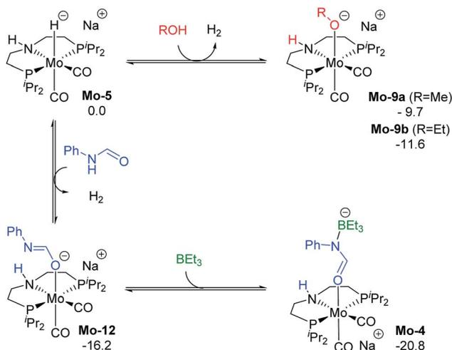
Scheme 6 Calculated Gibbs energies (kcal mol<sup>-1</sup>) for the substitution of H<sub>2</sub> in **Mo-5** by methanol, ethanol, formanilide and BEt<sub>3</sub> yielding **Mo-9a**, **b**, **Mo-10** and **Mo-4**, respectively.
