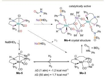
Scheme 5 Reactions performed to get insight on the active catalytic species (in dashed arrows) with the experimental observed products (H<sub>2</sub> and the crystal structure of Mo-4, in color) and the intermediates proposed (Mo-3 and Mo-5). Gibbs energies calculated for the dehydrogenation of Mo-5 at different pressure.
