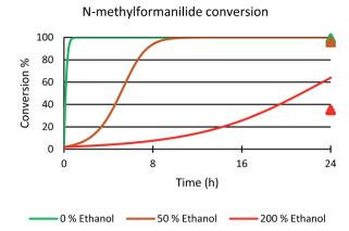
Fig. 7 Microkinetic simulation of *N*-methylformanilide **1a** conversion with 0% (green), 50% (brown) and 200% (red) ethanol in solution. The initial concentration of reactants were the same as those used in the experiments; *i.e.* 0.25 M *N*-methylformanilide **1a**, 0.207 M of dihydrogen and 12.5 mM of **Mo-5**. Experimental values at 24 hours represented with triangles.
