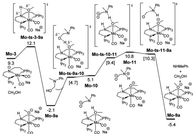
Fig. 5 Reaction pathway of the MeOH assisted hemiaminal proton transfer and posterior C–N bond cleavage. Gibbs energies in toluene (SMD) at 50 atm and 373 K are given in kcal mol<sup>-1</sup>.
