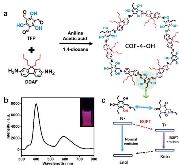
**Scheme 1** (a) The design of COFs to reveal the effects of hydroxyl and alkyl groups and the ESIPT procedure, showing hydroxyl-functional TFP and alkyl groups-containing DDAF for the preparation of COF-4-OH. (b) Dual emission from COF-4-OH under 280 nm excitation; inset: a picture of COF-4-OH under 280 nm illumination. (c) The ESIPT dual emission mechanism of hydroxyl-containing COF-4-OH.
