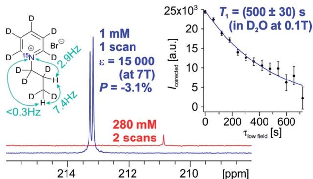
Fig. 1 Hyperpolarized  $^{15}\text{N}$  spectrum of **1a** (blue) by using PHIP in  $\text{D}_2\text{O}$  and thermally polarized  $^{15}\text{N}$  spectrum of the unsaturated precursor **1** (red) at 7 T. The inset shows the  $^{15}\text{N}$ - $T_1$  relaxation data measured at 0.1 T, using a hyperpolarized sample of **1a** which was collected using sample shuttling and small flip angle pulses (see ESI† for further details).
