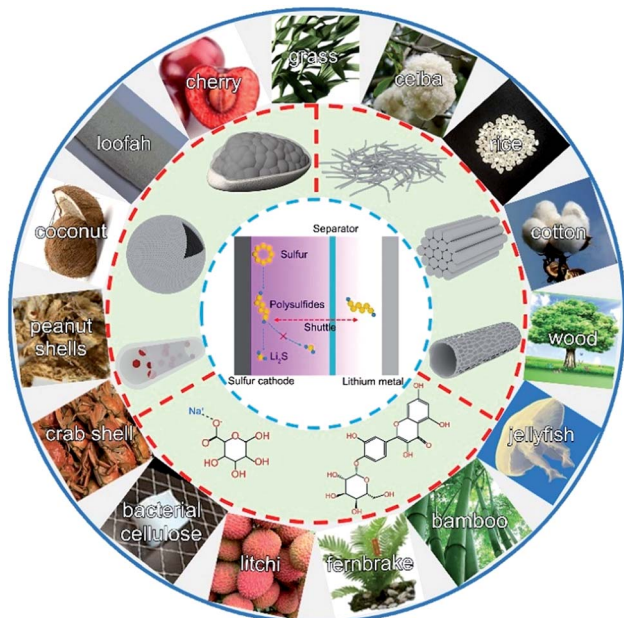
Fig. 1 The schematic diagram of bio-derived materials applied in the Li-S battery system.
