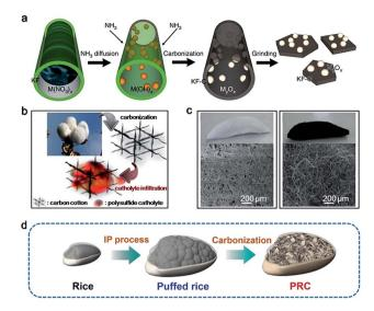
Fig. 2 (a) Fabrication diagram of  $M_xO_y/C$  composites. Reproduced with permission. Copyright 2016, Nature publishing group. (b) Schematic of the fabrication process of carbonized cotton. (c) Digital and SEM images of cotton and carbonized cotton. Reproduced with permission. Copyright 2016, American Chemical Society. (d) Schematic illustration of PRC. Reproduced with permission. Copyright 2017, Wiley-VCH.
