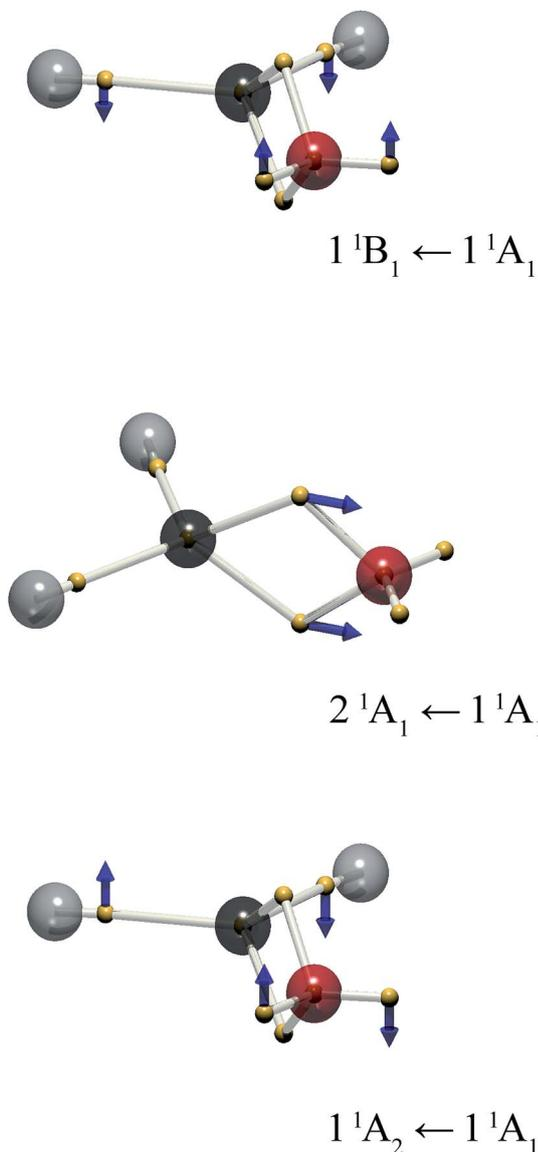
Fig. 4 The electron positions for the mid-point of the vibration,  $\bar{x} = (\bar{x}_i + \bar{x}_j)/2$ , and the displacement vectors  $x_{fi}$  for the wavefunction mixed between the  $1^1A_1$  (ground), and  $1^1A_2$ ,  $2^1A_1$  and  $1^1B_1$  excited states of formaldehyde. The vector length is doubled for clarity.
