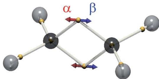
Fig. 3 The electron positions for the mid-point of the vibration,  $\bar{x} = (\bar{x}_i + \bar{x}_j)/2$ , and the displacement vector  $x_{fi}$  for the wavefunction mixed between the  $S_0$  and  $T_1$  states of ethylene. The  $\alpha$  and  $\beta$  electrons oscillate out of phase about the same midpoint, so there is no transition dipole moment.
