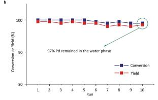
Fig. 4 (a) Conversions and yields of SM cross-couplings between bromobenzene and 4-methoxybenzeneboronic acid with pre-catalysts 6a, 6b, 6c and 6d. (b) Conversions and yields of target product (4-methoxybiphenyl) for the catalyst recycling experiments with 6a. Conversions and yields were determined using GC analysis.
