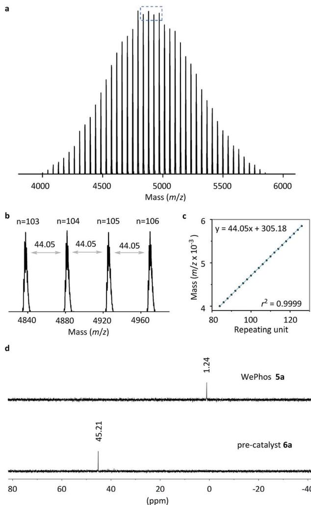
Fig. 2 (a) MALDI-TOF mass spectrum of WePhos<sub>5000</sub> **5a**. (b) Magnified MALDI-TOF mass spectrum of the blue box in (a). (c)  $m/z$  versus the number of repeating units for the MALDI-TOF mass spectrum of **5a**. (d) <sup>31</sup>P-NMR spectra of **5a** and **6a**.
