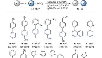
Scheme 4 Cross-coupling of (hetero)arvl chlorides with pre-catalyst **6a**. Conditions:  $R^1$ -X (0.5 mmol),  $R^2$ -B(OH)<sub>2</sub> (0.55 mmol), **6a** (50–500 ppm), K<sub>2</sub>CO<sub>3</sub> (1.0 mmol), H<sub>2</sub>O (0.8 mL), toluene (0.2 mL), 90 °C, 2 h. Catalyst loadings are listed in parentheses. Isolated yields are based on aryl chlorides. a5 h.
