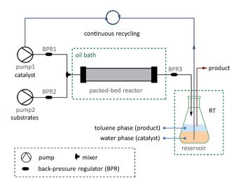
Fig. 5 Set-up for continuous catalyst-recycling synthesis based on flow chemistry.
