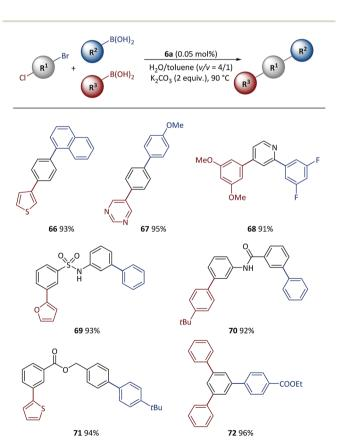
Scheme 6 Tandem SM cross-coupling with pre-catalyst **6a**. Conditions:  $R^1$ -X (0.5 mmol),  $R^2$ -B(OH)<sub>2</sub> (0.51 mmol),  $R^3$ -B(OH)<sub>2</sub> (0.55 mmol), **6a** (500 ppm),  $K_2$ CO<sub>3</sub> (1.0 mmol),  $H_2$ O (0.8 mL), toluene (0.2 mL), 90 °C. Isolated yields based on conjunctive dihalide compounds.
