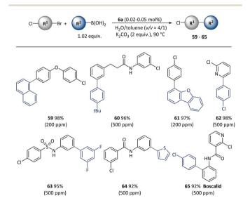
Scheme 5 The chemoselective cross-coupling of conjunctive dihalide compounds using pre-catalyst 6a. Conditions: Cl-R<sup>1</sup>-Br (0.5 mmol),  $R^2$ -B(OH)<sub>2</sub> (0.51 mmol), **6a** (50–500 ppm),  $K_2CO_3$  (1.0 mmol), H<sub>2</sub>O (0.8 mL), toluene (0.2 mL), 90 °C, 2 h. Catalyst loadings are listed in parentheses. Isolated yields are based on conjunctive dihalide compounds.
