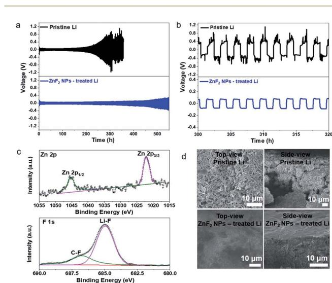
**Fig. 3** (a) The evolution of voltage profiles of symmetric cells based on the pristine Li metal anode (top) and ZnF<sub>2</sub> NPs – treated Li metal anodes (bottom), respectively. (b) The corresponding voltage profiles of (a) in an enlarged view of 300–320 h. (c) The Zn 2p, F 1s XPS spectra of the ASEI layer formed on Li foil after the 10th cycle. (d) The surface and side-view SEM images of the pristine Li metal anode and ZnF<sub>2</sub> NPs – treated Li metal anodes after 320 h cycling.
