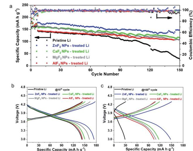
Fig. 4 (a) Electrochemical cycling performance at 0.5C and (b and c) representative charge/discharge profiles of cells based on the pristine Li metal anode and MF<sub>x</sub> NPs – treated Li metal anodes in the 10<sup>th</sup> and 150<sup>th</sup> cycle, respectively.
