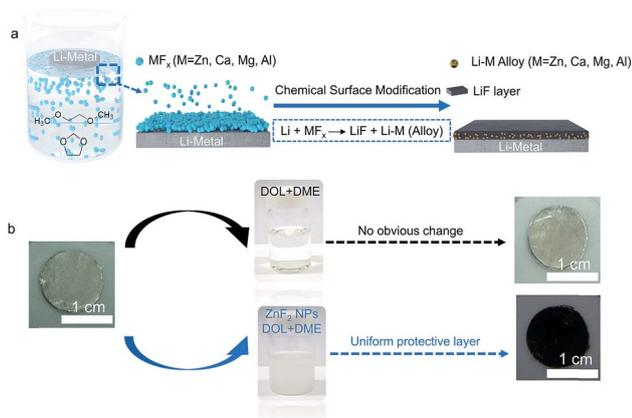
Fig. 1 (a) Schematic illustration of the ASEI layer formation *via ex situ* chemical modification. (b) Optical photographs of Li foil treated with co-solvent (DOL/DME) and co-solvent dispersed ZnF<sub>2</sub> NPs, respectively.
