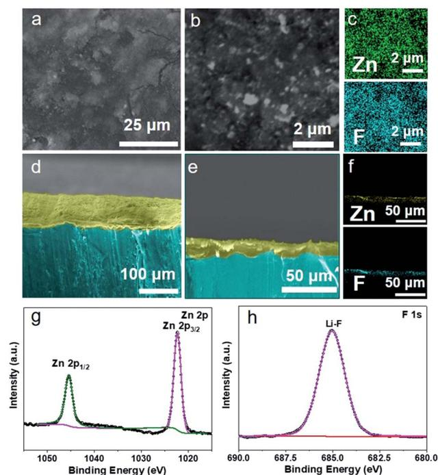
Fig. 2 (a and b) The top-view SEM images, (c) corresponding EDX mapping analysis, (d and e) side-view SEM images and (f) corresponding EDX mapping analysis of ZnF<sub>2</sub> NPs – treated Li metal anodes, respectively. The modified layer is denoted by cyan colour and the Li is denoted by green colour. (g and h) The Zn 2p, F 1s XPS analysis of the corresponding ASEI layer.
