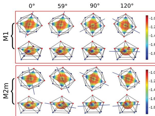
Fig. 6 Electrostatic potential computed by CAMMEL for **M1** and **M2m** at different  $\alpha$  angles. For each  $\alpha$  angle, the top and side views of the complex are shown. Only the atoms directly bonded to the Dy(III) ion are shown. Oxygen and nitrogen atoms are red and blue, respectively. The orientation (blue line) of the easy axis of magnetization for each geometry is also shown.
