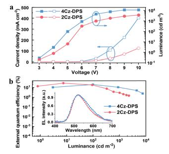
4 (a) Current density-voltage-luminance and (b) external quantum efficiency-luminance curves of 4Cz-DPS and 2Cz-DPS devices. Inset: normalized EL spectra.
