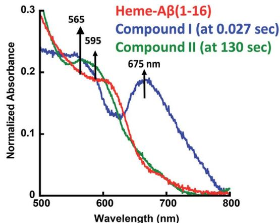
Fig. 1 Absorption spectrum of heme- $\text{A}\beta$ (1–16), red; for the reaction of heme- $\text{A}\beta$ (1–16) with *m*-CPBA in 50 mM  $\text{PO}_4^{3-}$  buffer at pH 8, the difference spectrum at 0.027 s (compound I), blue; and the difference spectrum at 130 s (compound II), green. The arrows indicate the direction of the spectral changes. A difference spectrum at a given time is the difference between the spectrum at that time and the spectrum of initial heme- $\text{A}\beta$ .
