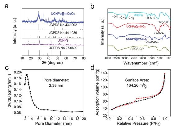
Fig. 2 XRD patterns of UCNPs and UCNPs@mCeO<sub>x</sub> (the standard lines of  $\beta$ -NaGdF<sub>4</sub>, CeO<sub>2</sub> and Ce<sub>2</sub>O<sub>3</sub> are supplied for comparison) (a) and FT-IR spectra of OA-UCNPs, UCNPs@mSiO<sub>2</sub>, UCNPs@mCeO<sub>x</sub> and PEG/UCP (b). The pore-size distribution (c) and N<sub>2</sub> adsorption/desorption isotherm (d) of UCNPs@mCeO<sub>x</sub>.
