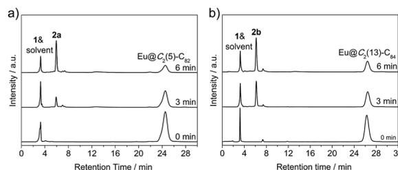
Fig. 1 HPLC profiles of the reaction mixture containing **1** and (a)  $\text{Eu}@C_2(5)\text{-C}_{82}$  or (b)  $\text{Eu}@C_2(13)\text{-C}_{84}$  probed at different reaction times. HPLC conditions: Buckyprep column ( $\phi = 4.6 \times 250$  mm); 20  $\mu\text{L}$  injection volume; 1.0  $\text{mL min}^{-1}$  toluene flow; 40  $^\circ\text{C}$ ; 330 nm detection wavelength.
