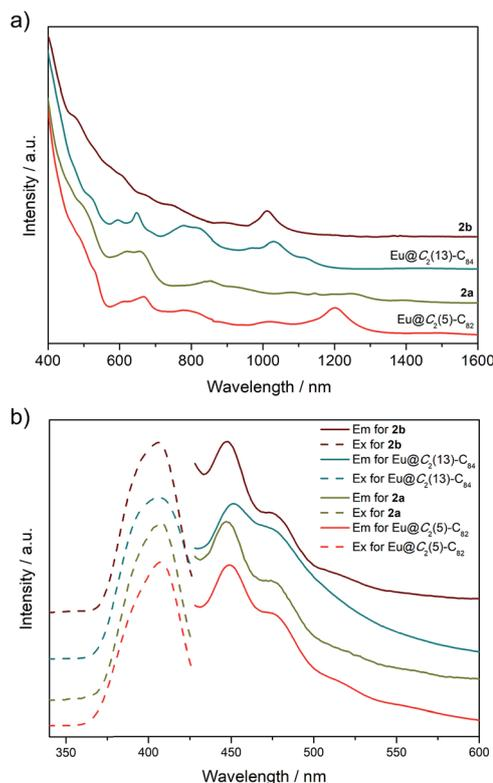
Fig. 2 (a) Vis-NIR absorption spectra and (b) photoluminescence emission and excitation spectra of  $\text{Eu}@C_2(5)\text{-C}_{82}$ , **2a**,  $\text{Eu}@C_2(13)\text{-C}_{84}$  and **2b** dissolved in  $\text{CS}_2$  at room temperature. The curves are vertically shifted for ease of comparison.
