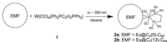
Scheme 1 Reaction of **1** with  $\text{Eu}@C_2(5)\text{-C}_{82}$  or  $\text{Eu}@C_2(13)\text{-C}_{84}$ .
