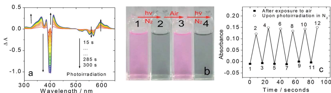
Fig. 7 (a) UV-vis difference absorption spectra of 1PF 2 in the presence of Et 3 N in the deaerated MeCN with white light continuous photo-irradiation using a xenon lamp, light power density: 5.2 mW cm -2 . (b) Photos showing the consecutive color change of the 1PF 2 /Et 3 N mixed solution upon alternating photoirradiation and exposure to air: (1) Without photoirradiation under an air atmosphere; (2) Upon 8 second photoirradiation under a N 2 atmosphere; (3) Exposure to air after photoirradiation; (4) Upon another 8 second photoirradiation under a N 2 atmosphere. (c) Reversibility of the formation of 1PF 2 •- monitored at the 594 nm absorption band (after generation of 1PF 2 •- , re-exposure to air will oxidize the radical anion to the neutral form 1PF 2 ). Photoirradiation power density is 23 mW cm -2 . c [ 1PF 2 ] = 1 × 10 -5 M and c [Et 3 N] = 0.25 M, 20 °C.
