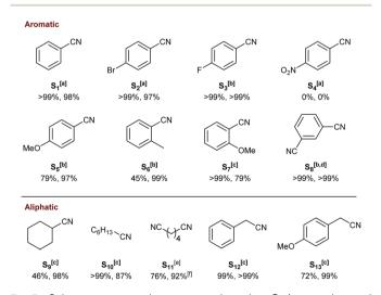
Fig. 5 Substrate scope using supported catalyst  $C_1$  (conversion and selectivity to mono- or diamine indicated below structures). <sup>a</sup>Reaction conditions: substrate (0.5 mmol), [Ru] (1.0 mol%), dioxane (1.0 mL), 80 °C, H<sub>2</sub> (10 bar), 18 h. <sup>b</sup>100 °C. <sup>c</sup>120 °C. <sup>d</sup>H<sub>2</sub> (30 bar), 24 h. <sup>f</sup>Selectivity towards ω-aminocapronitrile.
