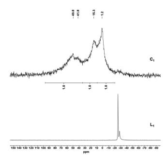
Fig. 3  $^{31}$ P NMR (THF) monitoring of the representative SPS of supported Ru–Triphos complex C<sub>1</sub>.
