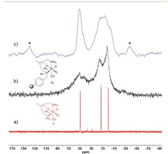
Fig. 4 (a)  $^{31}P$  NMR spectrum of solution-phase analogue 3, (b) gelphase  $^{31}P$  NMR spectrum of supported complex  $C_1$  and (c) solid-state  $^{31}P$  MAS NMR spectrum of  $C_1$ . Rotational sidebands are denoted by asterisks (\*).
