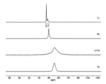
Fig. 2  $\,\,^{31}\text{P}$  NMR (THF) monitoring of the representative SPS of supported Triphos-ligand  $L_1.$
