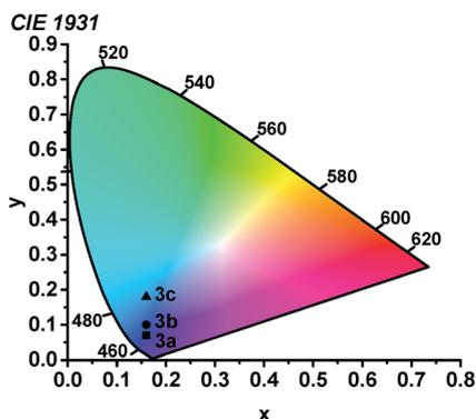
Fig. 6 Chromaticity diagram showing the (CIE<sub>x</sub>, CIE<sub>y</sub>) coordinates of **3a–c**.
