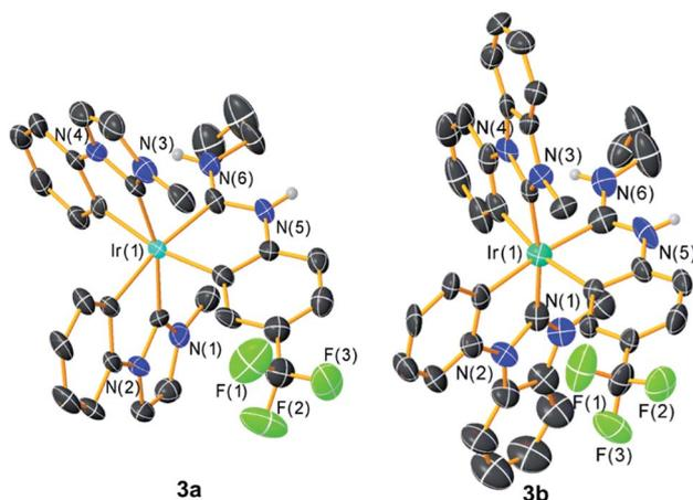
Fig. 2 Crystal structures of complexes **3a** and **3b**, with ellipsoids shown at the 50% probability level. Carbon atoms are shown in black and unlabeled, and carbon-bound hydrogen atoms are omitted for clarity.
