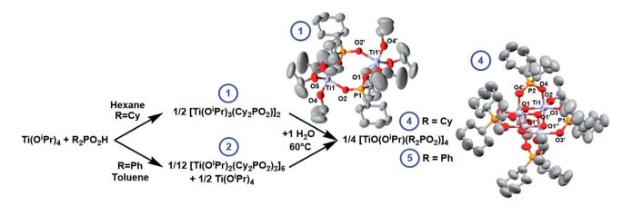
Fig. 2 Reaction of  $Ti(O^iPr)_4$  with  $R_2PO_2H$  and subsequent hydrolysis, with solid-state structures of **1** and **4**, hydrogen atoms omitted for clarity. Ellipsoids displayed at 50% probability. Selected bond lengths (Å) and angles (°) **1**: P1-O1, 1.5054(17); P1-O2, 1.5260(17); P1-O1, 2.0050(16); P1-O1, 2.19837(16); P1-O1, 2.19837(16); P1-O1, 2.19837(16); P1-O1, 2.1912(2); P1-O1, 2.1912(2); P1-O1, 2.1912(2); P1-O1, 2.1913(3); P1-O1, 2.19
