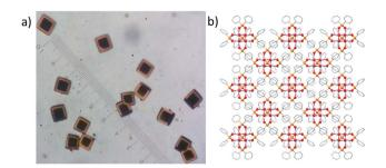
Fig. 9 (a) Oxidation of single crystals of 7 under air. Crystals undergo reaction from surface downwards. (b) Packing diagram of 7 (with phenyl groups in stick notation and hydrogen atoms omitted) showing symmetrical nature of the complex and possibility for incorporation of small anions within the lattice.
