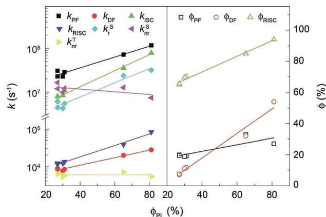
Fig. 5 Linear correlations between  $\phi_{\text{PL}}$  of 4ArDPDPO2A, 4ArPPOPO and 4ArPPDPO and the rate constants ( $k$ ) and efficiencies ( $\phi$ ) of the key transitions involved in the TADF process.
