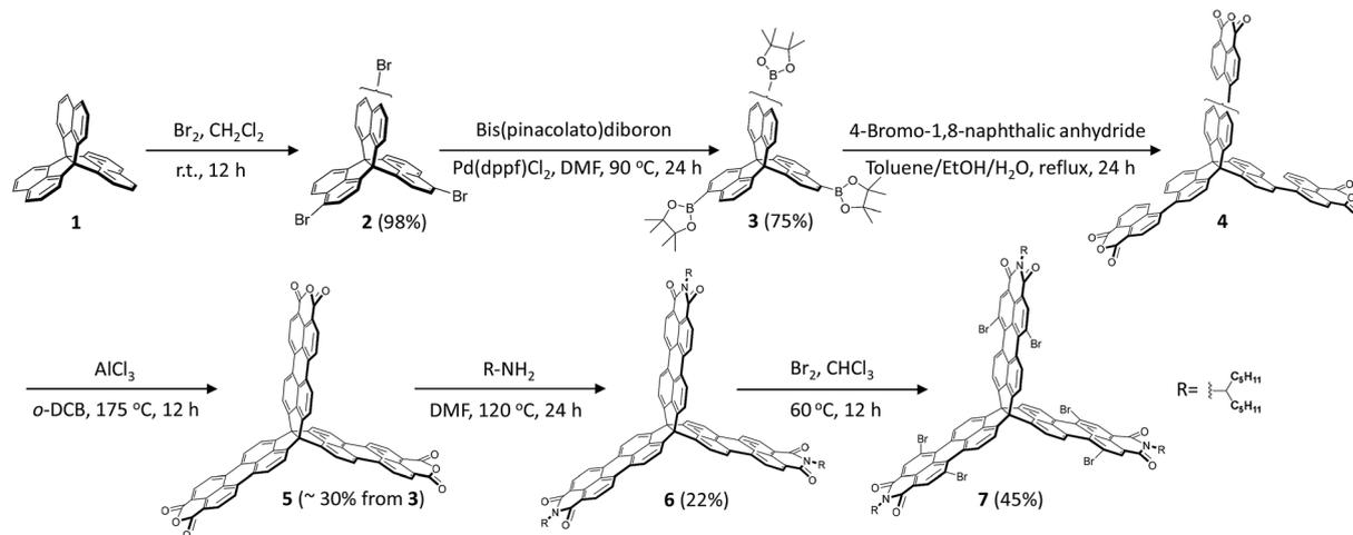
Scheme 1 Synthetic steps to 3D-symmetric building block **6** and its brominated **7**.
