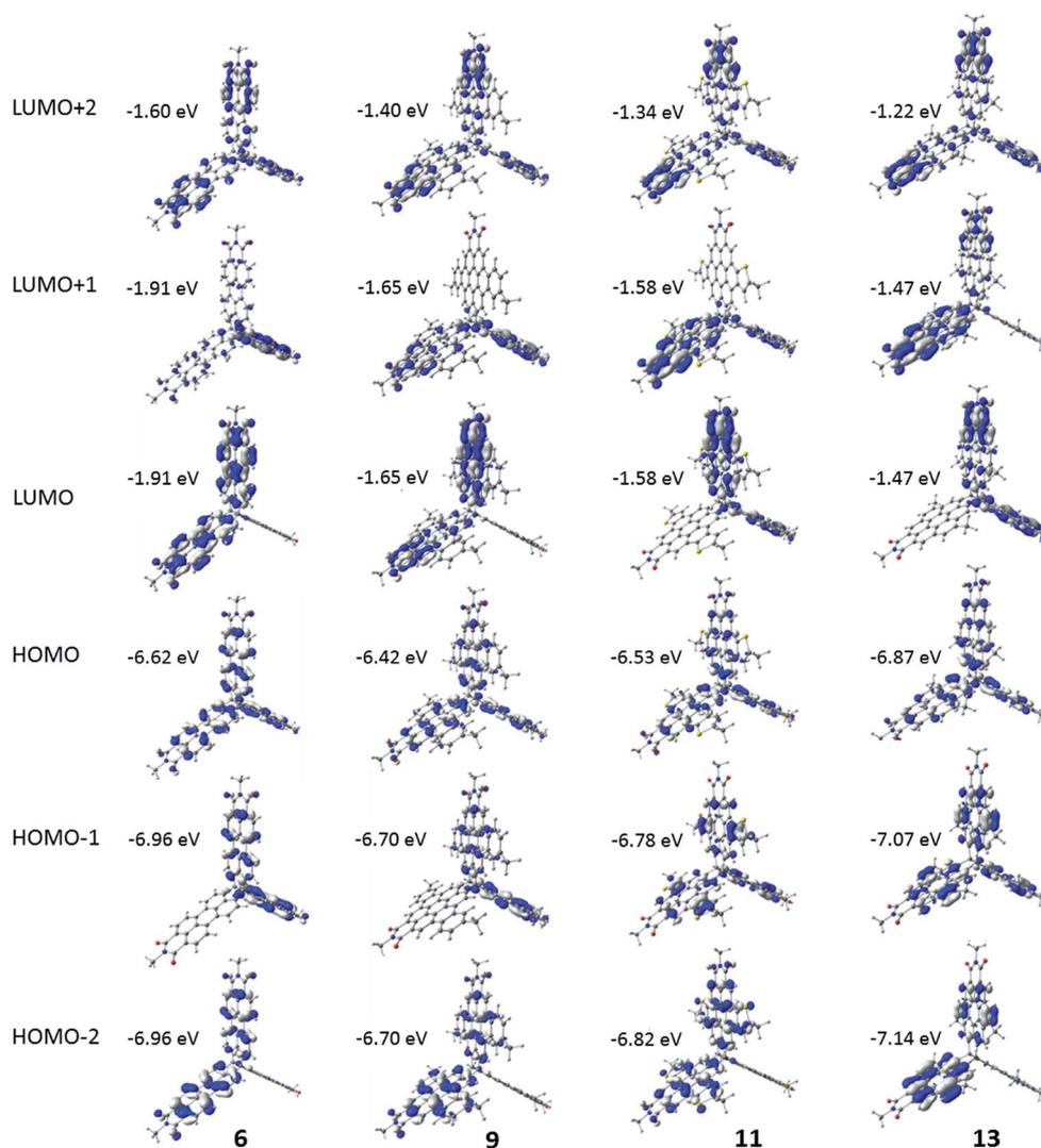
Fig. 3 Pictorial representations of selected frontier molecular orbitals of **6**, **9**, **11**, and **13** as determined at the OT- $\omega$ B97X-D/6-31g(d,p) level of theory. Pictorial representations of the monomeric units are shown in the ESI<sup>†</sup>.
