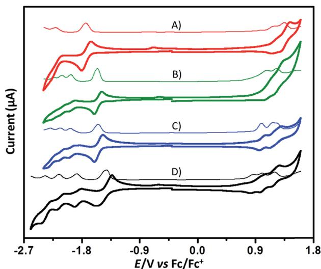
Fig. 5 Cyclic voltammograms (bold solid line) and differential pulse voltammograms (thin solid line) of **13** (A), **11** (B), **9** (C), and **6** (D), performed in nitrogen-purged dichloromethane with TBAPF<sub>6</sub> (0.1 M).
