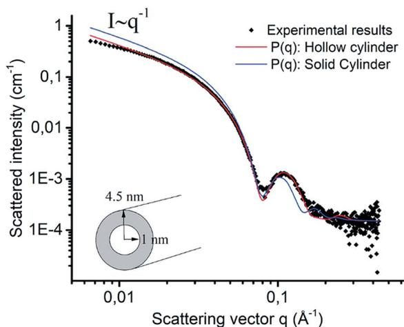
Fig. 2 SAXS scattered intensity plot against the scattering vector ( $q$ ) for  $[\text{ALV}]_3[\text{KGE}]_4$  assembled at  $5 \text{ mg mL}^{-1}$  in pH 4 buffer by direct dissolution (black) vs. the fitted model for solid (blue) and hollow (red) cylindrical shaped micelles.
