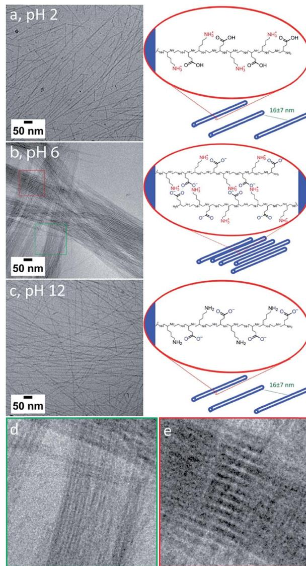
Fig. 4 CryoTEM images and schemes of  $[\text{ALV}]_3[\text{KGE}]_4$  assembled via direct dissolution at  $10 \text{ mg mL}^{-1}$  in pH 2 (a), 6 (b) and 12 (c) buffer. Zoom-in of (b) showing the bundled composition out of nanotubes (d) and an organization-induced interference pattern (e).
