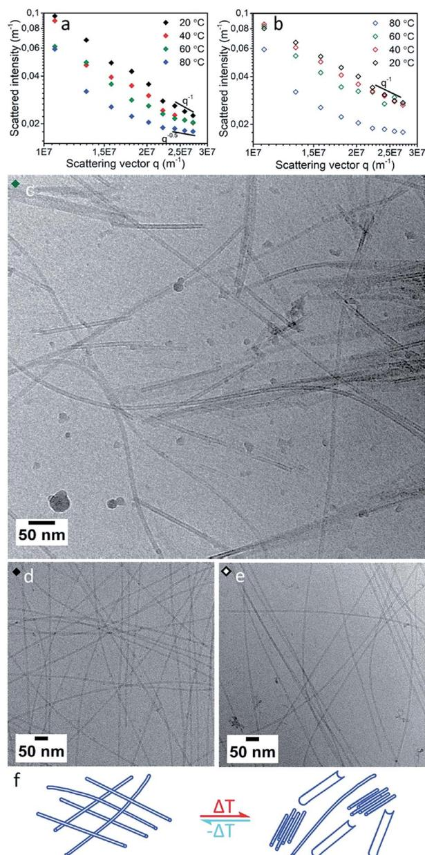
Fig. 3 SLS results for  $[\text{ALV}]_3[\text{KGE}]_4$  at  $0.5 \text{ mg mL}^{-1}$  in pH 4 buffer collected at 20, 40, 60 and 80 °C, during heating (a) and cooling (b). CryoTEM of  $[\text{ALV}]_3[\text{KGE}]_4$  heated to 58 °C during vitrification (c), before heating (d) and after the SLS heating procedure (e). Scheme of observed species (f) before/after heating (left) and during at  $\sim 60$  °C (right).
