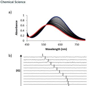
Fig. 3 (a) UV/Vis absorption spectra for titration of 24 into 1 (0.2 mM) in acetonitrile at 298 K. The initial spectrum of unbound 1 is shown in blue, and the final spectrum corresponding to the bound complex  $1\cdot24$  is shown in red. (b) 162 MHz  $^{31}$ P NMR spectra for titration of 24 into 2 (6 mM) in acetonitrile at 298 K.
