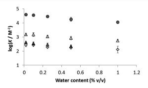
Fig. 4 Effect of added water on association constants measured in acetonitrile (shaded) and acetone (open): 1.8 circles, 1.26 triangles and 1.14 diamonds. The water content of both solvents without addition of water is 0.02%.
