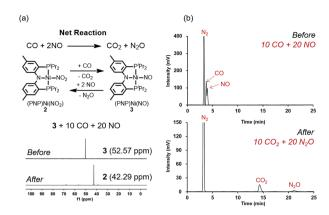
Fig. 9 (a) Schematic representation of catalytic reaction to convert CO and NO to CO<sub>2</sub> and N<sub>2</sub>O (top). <sup>31</sup>P NMR spectra of **3** and its reaction with 10 equiv. of CO and 20 equiv. of NO in  $C_6D_6$  at room temperature (bottom). (b) Gas chromatogram of the headspace gases converted during the reaction of **3** with 10 equiv. of CO and 20 equiv. of NO.
