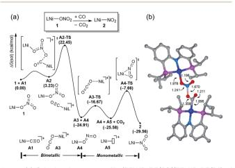
Fig. 4 (a) Calculated energy profile (B3LYP-D3/B2//B3LYP-D3/B1) of the bimetallic pathway from  $\bf 1$  to  $\bf 2$ . (b) The computed structure of the transition state A2-TS. Non-essential atoms are not shown for clarity. All distances are given in  $\dot{\bf A}$ .
