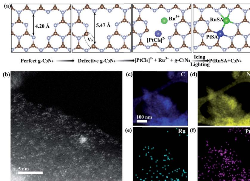
Fig. 1 (a) Schematic illustration of the icing-assisted *in situ* photocatalytic reduction method for preparing PtRuSA–CN620. (b) HAADF-STEM images of PtRuSA–CN620 and the corresponding distribution of (c) C, (d) N, (e) Ru and (f) Pt. Scale bar: 5 nm.
