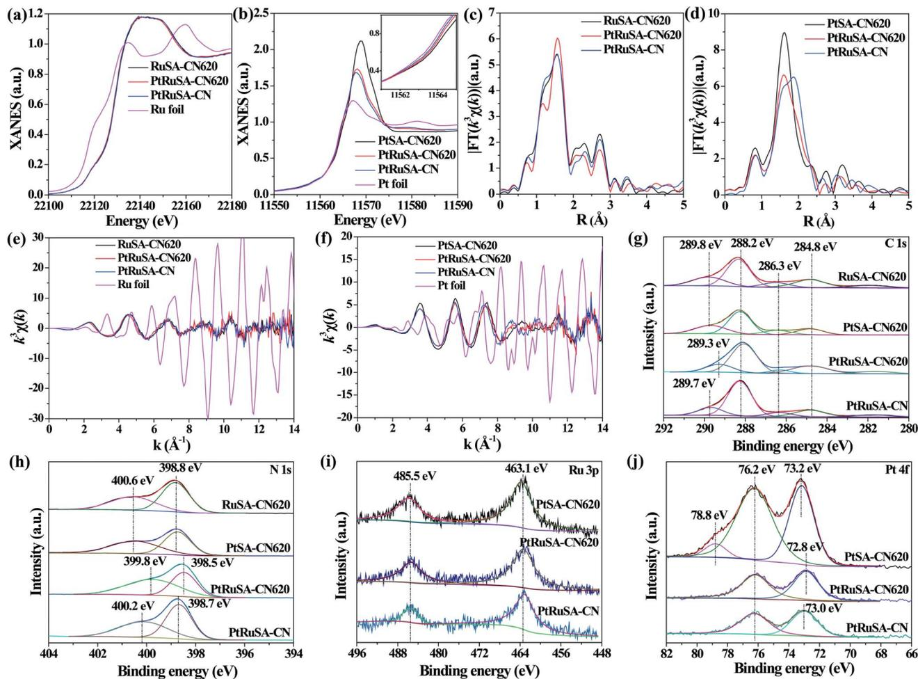
Fig. 2 (a) Ru K-edge and (b) Pt  $L_{3}$ -edge XANES spectra of as-prepared samples and the corresponding  $k^3$ -weighted FT spectra of Ru and Pt at (c and d)  $R$  space and (e and f)  $k$  space. XPS survey spectra of (g) C 1s, (h) N 1s, (i) Ru 3p and (j) Pt 4f of as-prepared samples.
