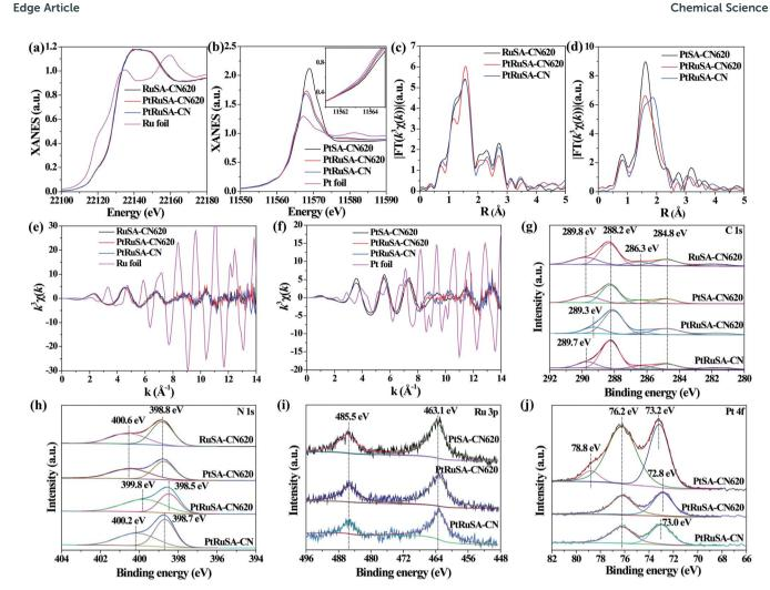
Fig. 2 (a) Ru K-edge and (b) Pt  $L_3$ -edge XANES spectra of as-prepared samples and the corresponding  $k^3$ -weighted FT spectra of Ru and Pt at (c and d) R space and (e and f) k space. XPS survey spectra of (g) C 1s, (h) N 1s, (i) Ru 3p and (j) Pt 4f of as-prepared samples.
