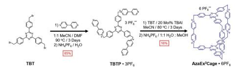
Scheme 1 Synthesis of AzaEx<sup>2</sup>Cage · 6PF<sub>6</sub> from TBT.
