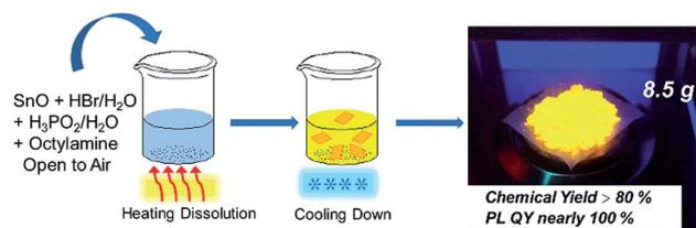
**Scheme 1** Schematic representation of the synthesis of the 2D (OCTAm)<sub>2</sub>SnBr<sub>4</sub> by a facile aqueous acid-based synthetic method in ambient air.
