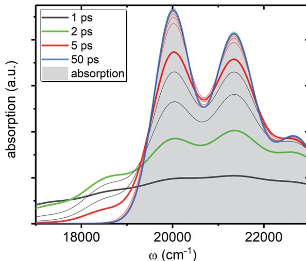
Fig. 5 IA component,  $A_A(\omega, t)$ , from the ground state of the artificial system. All parameters are the same as in Fig. 4c. The shaded contour shows  $A_A(\omega, \infty)$ , which is the absorption spectrum of the artificial system. The faint gray lines correspond to spectra separated by 1 ps time step, while the faint red lines correspond to 10 ps time step, starting from 10 ps.
