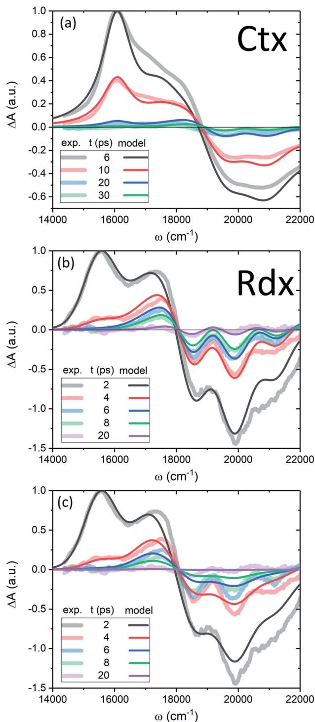
Fig. 7 (a, b) TA of Ctx and Rdx, accordingly. Thick-faint lines correspond to measurements, thin lines represent the model fitting. (c) TA of Rdx without the line-width dependence on temperature ( $\eta = 0$ ).
