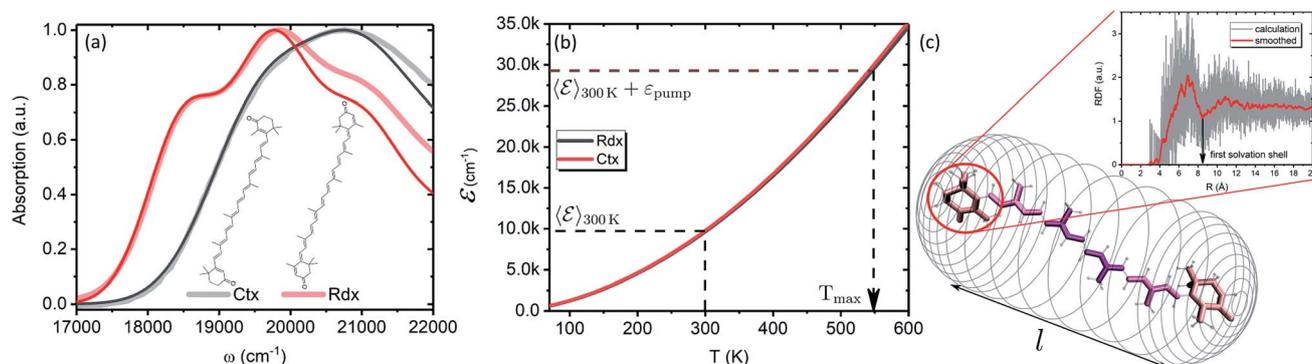
Fig. 6 (a) Absorption spectra of Ctx and Rdx in benzene. Thick-faint lines correspond to the measurement, thin lines represent fitting. (b) Internal energy as function of temperature. (c) Schematic representation of the FSS as a cylindrical mesh. Highlighted are the segments of a carotenoid chosen for RDF calculation. The inset shows RDF of an end group of Ctx as obtained from the MD simulation. Red line corresponds to the Savitzky–Golay smoothing for the extraction of FSS radius.
