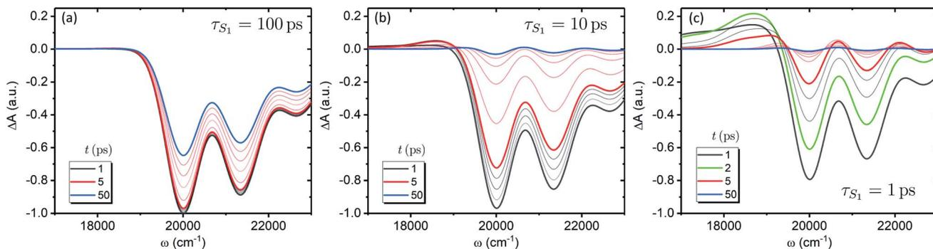
Fig. 4 TA spectra of the artificial system. Panels a to c correspond to the  $|S_1\rangle$  state lifetimes of 100, 10 and 1 ps, accordingly. All the spectra are normalized to the maximum level of the spectrum at 1 ps for the  $\tau_{S_1} = 100$  ps parameter set (panel a). The faint gray lines correspond to spectra separated by 1 ps time step, while the faint red lines correspond to 10 ps time step, starting from 10 ps.
