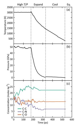
Fig. 1 Time histories for the (a) temperature, (b) pressure, and (c) concentration of C–C, C–N, and C–O bonds during a typical simulation as the system passes through high temperature and pressure, adiabatic expansion, cool down, and equilibration stages. Start and end times for each stage are shown with dashed lines. All plotted quantities were block averaged in contiguous non-overlapping 5 ps windows.
