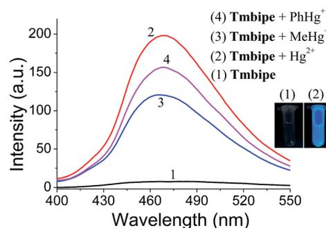
**Fig. 1** Fluorescence spectra of **Tmbipe** in the absence and presence of  $\text{Hg}^{2+}$ ,  $\text{MeHg}^+$  or  $\text{PhHg}^+$ . [**Tmbipe**] = 10  $\mu\text{M}$ ; [ $\text{Hg}^{2+}$ ] = [ $\text{MeHg}^+$ ] = [ $\text{PhHg}^+$ ] = 20  $\mu\text{M}$ . The inset shows the aqueous solution photograph of **Tmbipe** in the absence and presence of  $\text{Hg}^{2+}$  under UV light irradiation.
