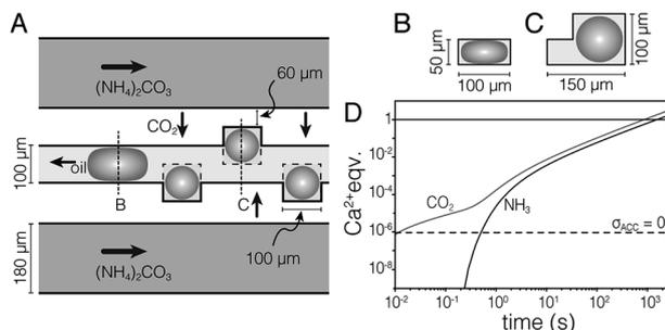
**Fig. 1** (A) Schematic drawing of the droplet orchard device. In the oil channel, droplets take an ellipsoidal shape (B), but can relax on entering the wells (C). (D) Plot of stoichiometric equivalents of CO<sub>2</sub> and NH<sub>3</sub> delivered to the droplet versus time, predicted by finite element modeling. Droplets are supersaturated for ACC ( $pK_{sp} = 6.04$ , ref. 21) the dashed horizontal line.
